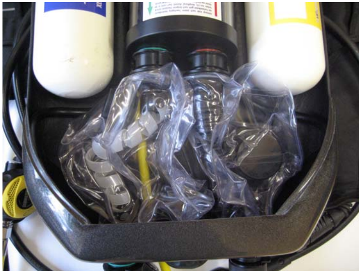
Low-pressure test breathing loop (separate breathing bags)
