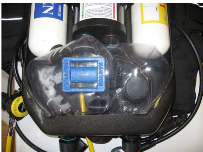
Overpressure test breathing loop (separate breathing bags)
