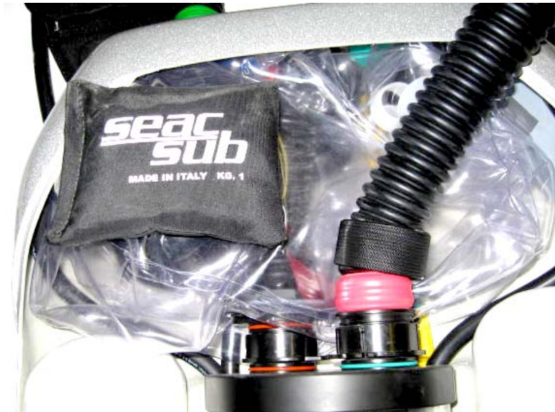
Sealing of the scrubber tank with the breathing hose (coaxiale breathing bags)
