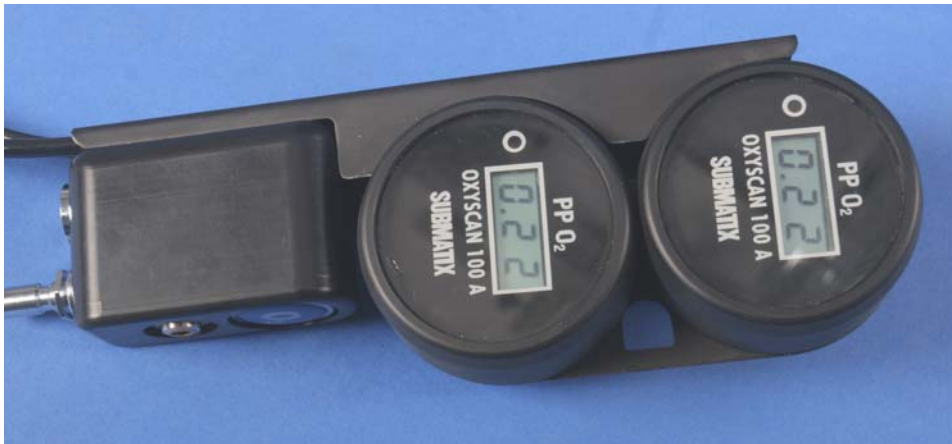
ppO 2 -monitoring system (Oxyscan), console mounted with gas booster
