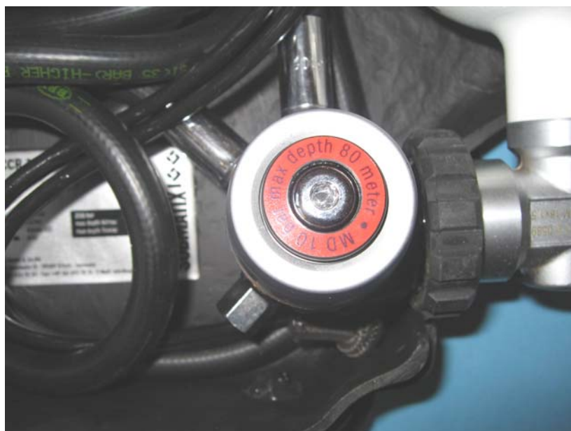
Pressure reducer Oxygen with overpressure valve and label factory settings 10 bar/80 m
