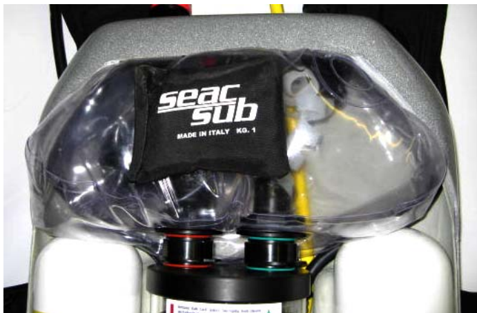
Overpressure test breathing loop (coaxiale breathing bags)
