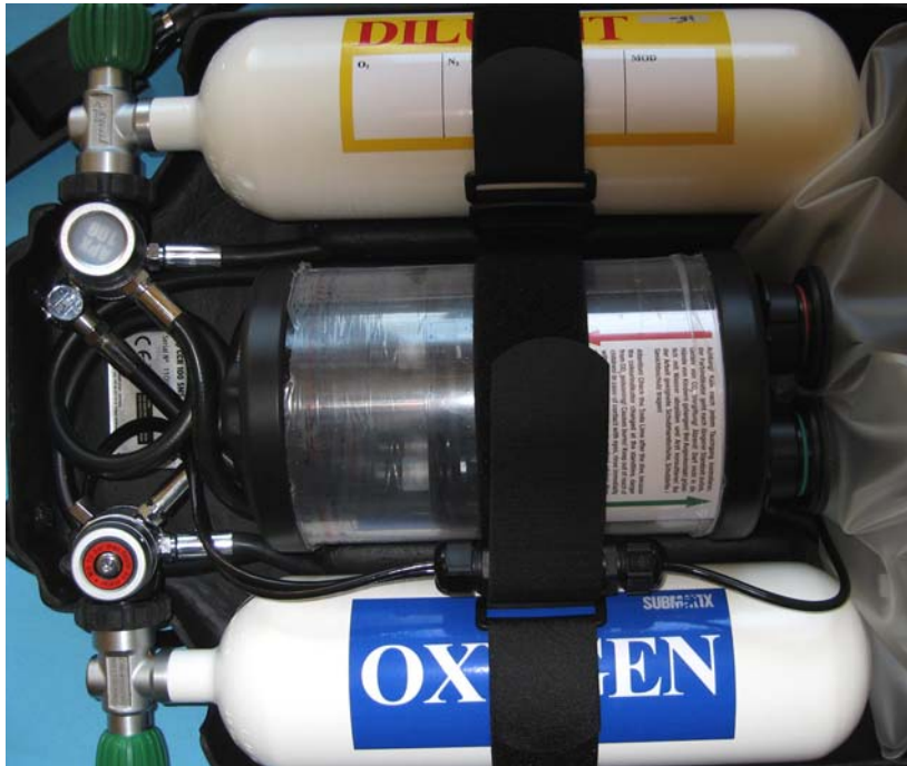
Gas supply: below: Oxygen, above: Diluent
