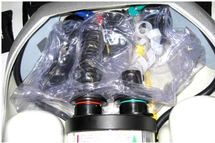
Low-pressure test breathing loop (coaxiale breathing bags)
