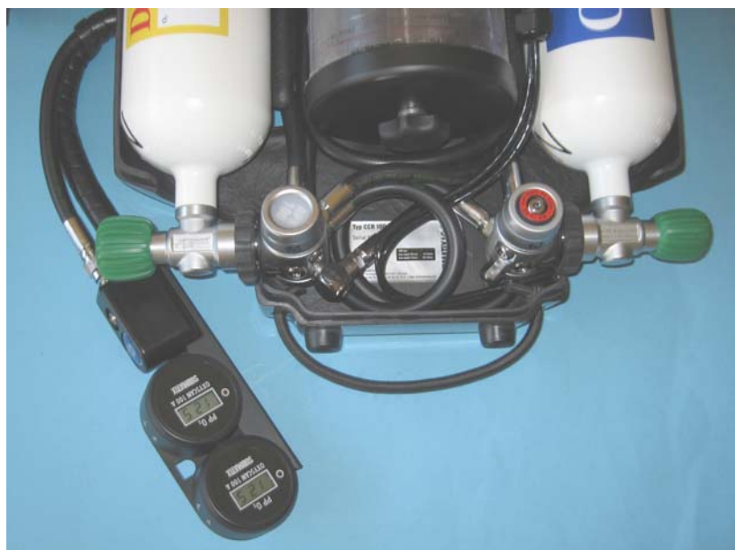
Gas supply: right: oxygen tank with fixed first stage, left: diluent tank with depth compensated first stage, below: gas booster with adjustable needle valve and quick-release coupling, console mounted with 2 x Oxyscan 100 Pro A
