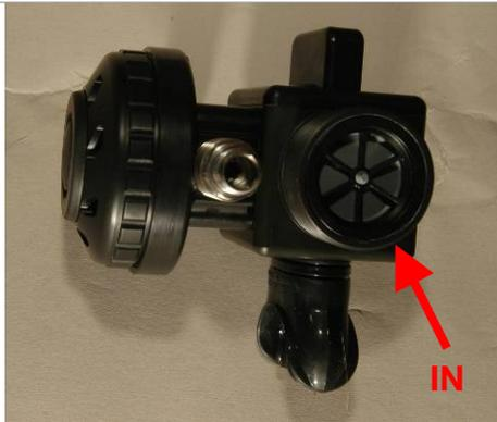
The gas will travel into the flapper valve in which the spokes are visible, and out of the valve with rubber flapper on top.
