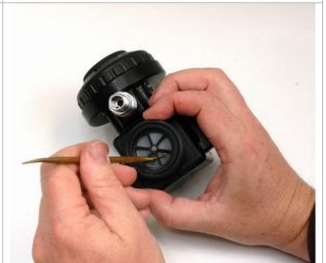
On the exhalation side, lift the flapper valve to reach the holder spokes.
