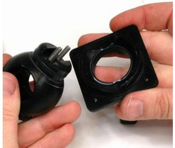
Inspect o-ring on the valve cover.
