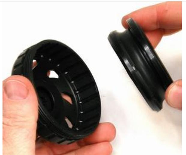
**Make sure that the diaphragm is seated properly, and that there is an o-ring on the circumference. The center of the diaphragm must be seated in the center of the purge button on the 2<sup>nd</sup> stage cover**
