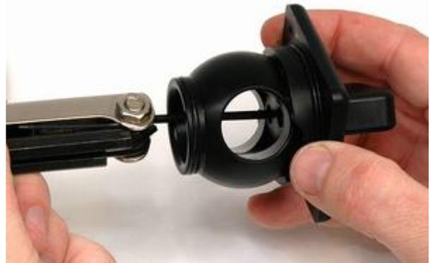
Separate the ball valve from the valve cover.
