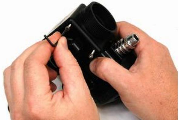
Pull the ball cover (and the ball valve) out of the BOV body. Make sure that BOTH retaining washers from the inhalation and exhalation ports are removed, otherwise you will not be able to remove the ball valve, and might damage the BOV.
