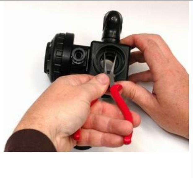
Alternatively, you can use the hook to pull on one of the holes of the retaining washer and twist it out of the groove. Remove retaining washer on the other side as well.
