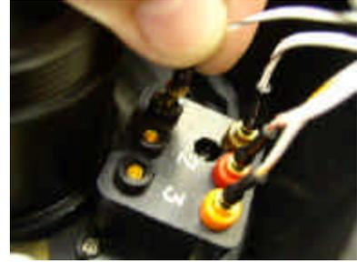
The next task is to connect the sensors, connect the brown cable to sensor 1, the red cable to sensor 2 and the orange cable to sensor 3. Be careful about the polarity of these wires – if any Sensor is reading “zero” on your Primary or Secondary, the black (common) wire and one or more of the colored striped wires are probably reversed at the banana block. The sensors use three pin connectors, **Molex P/N 22-01-3037**, which can only be connected only one way.
