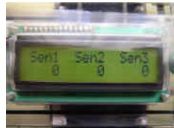
**drain the battery.** Pressing either button will exit this test. The output of each of the three main sensors should be recorded while in both AIR and Oxygen.
