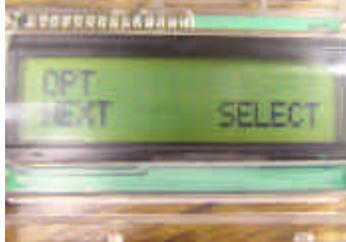
The next set of options is entered through the "OPT" menu. Selecting this screen enters a sub-menu containing programming, calibration, and testing options. Some options will be locked out once the Wrist Unit enters dive mode.
