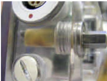
The picture to the left shows typical corrosion of the switch assembly. This is usually the result of salt-water residue in the switch cavity and can usually be prevented by proper rinsing. This switch will be disassembled to inspect, clean and replace components if necessary.
