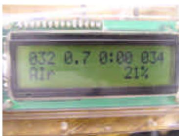
The final display may seem like an annoyance, but it serves as a reminder to the diver. The name of the diluent the diver has selected and the programmed Oxygen percentage of the diluent are displayed on the bottom line. This should help insure the diver doesn't try and use a nitrogen mix with same Oxygen percentage as a helium based gas.
