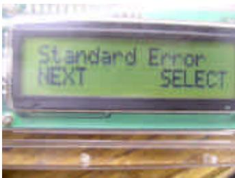
This option sets the allowable error before the solenoid fires in “Standard Mode”. The valid range is from 1% to 10%. A lower value is not necessarily a better setting. In shallow water, a low value will hold a stable set-point with little or no overshoot, but as depth increases, overshooting the set-point is
