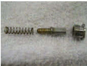
Even though the push button and spring are made out of stainless steel, corrosion can be seen on both parts. This is due to the reaction between the different stainless steel alloys used. The corrosion can be removed by placing the individual components in a diluted bath of common household vinegar for several minutes.
