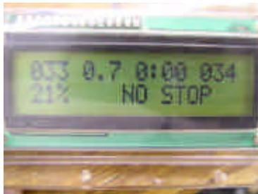
The next display depends on the status of the diver's decompression obligation. The top line is the same as on the previous screen with the change being on the second line. Instead of the PO<sub>2</sub> being displayed, the Oxygen percentage of the selected diluent and "No Stop" is displayed until the diver enters a required decompression stop.
