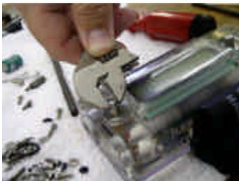
The first step is to loosen the boss assembly using an adjustable or 1/4 inch wrench. Do not use excessive force. Once the assembly is free, remove it from the Wrist Unit.
