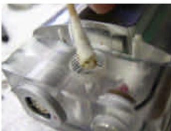
Clean out the compartment with a Q-Tip, lube the components with some silicon, and reassemble. The picture on the right shows the same compartment after cleaning.
