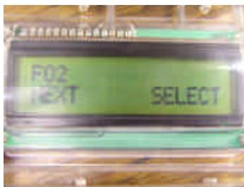
The next selection is the FO<sub>2</sub> display screen. Pressing the right button will immediately display the calculated PO<sub>2</sub> for the current diluent and current depth. A proper loop flush with diluent should result in this value.
