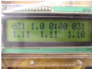
The next screen is the first of three displays presented while in dive mode. The top line displays current depth, chosen set-point, dive time and maximum depth. The bottom line displays the PO<sub>2</sub> readings of the three sensors as in the previous display. If any sensor reading is followed by a "\*" that sensor has been voted out and is not used in the average PO<sub>2</sub> calculation.
