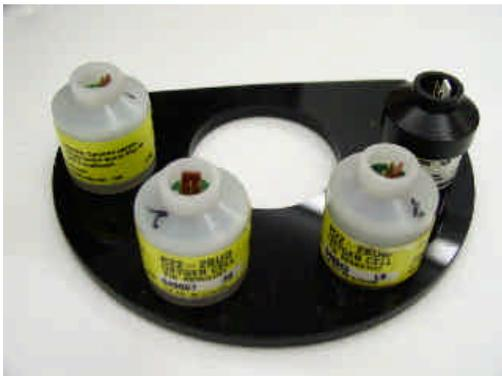
The last position is only used when an external PO<sub>2</sub> monitor or integrated dive computer is connected. The proper cable is available for the HS-Explorer and VR3 computers. The sensors should be installed such that the face is visible with the plate numbering on the outer edge. The sensors will work in either orientation but this arrangement permits easy identification while the plate is installed. The sensor o-ring should be removed
