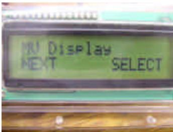
This option displays the calculated millivolt output on each of the three Oxygen sensors. All measurements are rounded to the nearest mV. **The backlight will remain illuminated and will not timeout. Failure to exit this test will**
