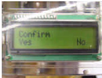
***All confirmations are made utilizing the left button. This was chosen to prevent accidental confirmations due to double key presses.***
