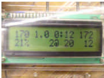
Once a decompression ceiling is present, the next display becomes active. The top line remains unchanged, while the bottom line displays the Oxygen percentage of the diluent, deepest stop depth and time, followed by the total ascent time. The sample screen shows the deepest stop at 20fsw for two minutes and a TTS of 12 minutes.
