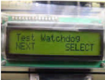
The “Test Watchdog” option performs a hard reset on the Wrist Unit. This action has the same effect as removing and replacing the battery/batteries.
