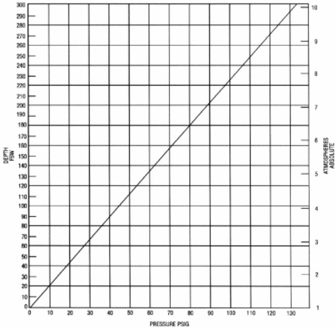
Figure 2-7. Depth, Pressure, Atmosphere Graph.
