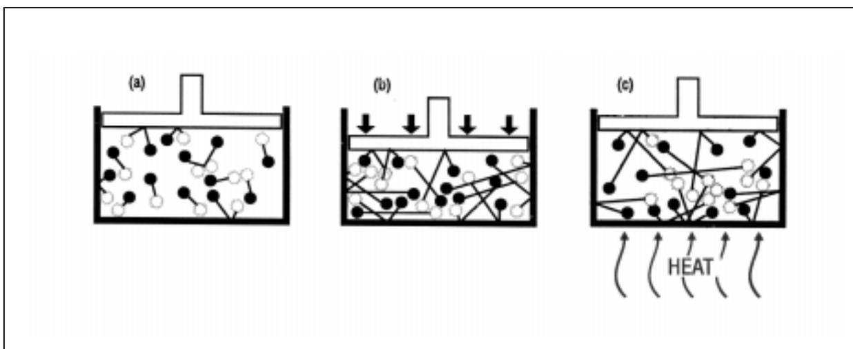
**Figure 2-6.** Kinetic Energy. The kinetic energy of the molecules inside the container (a) produces a constant pressure on the internal surfaces. As the container volume is decreased (b), the molecules per unit volume (density) increase and so does the pressure. As the energy level of the molecules increases from the addition of thermal energy (heat), so does the pressure (c).
