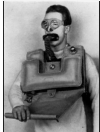
**Figure 1-10.** Original Davis Submerged Escape Apparatus.
